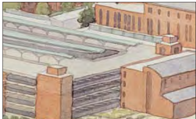
Plan Proposal – Use photovoltaic cells as shade devices and energy collectors on top of parking decks
